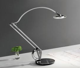
Product: Birdie Designer: Olle Lundberg Dimensions: 100x76x11 Materials: Lamp housing and arm in aluminium, footplate in steel. Available in graphite black, and white options. Light source: LED 7W, 511Im, 73Im/W. Samsung LED source, 3000K, RA min 80, <5 SDCM, 50,000 hours Features: Minimalistic design, high lumen output, intelligent slide dimmer 0 to 100%. Memory-stored settings
