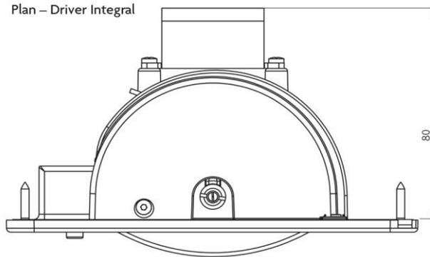
Should this depth be too great for the space available, the driver may be removed from the casing by loosening the retaining bolts and mounted remotely onto the back of the headboard or wall using the 2 x domed-head self-tapping 'twin-fast' screws provided. This option reduces the depth required to 58mm.
